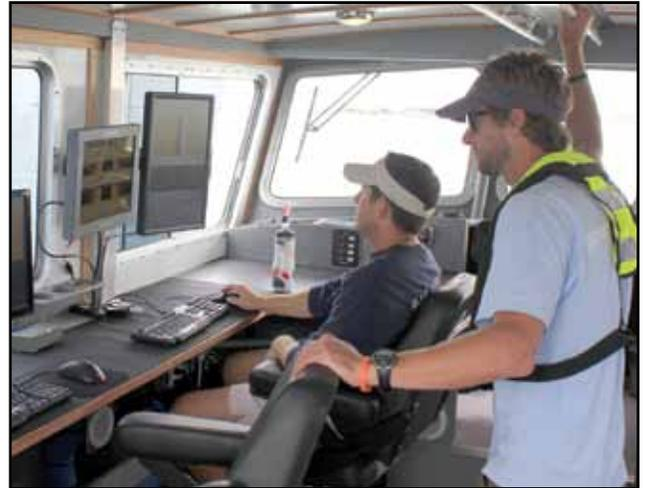
Hydrographic Surveyors Ben Sumners and David Bernstein (seated) collect both multibeam and sidescan sonar to NOAA and IHO specifications for the Port of Morehead City project to investigate conditions of the berths for ship clearance. The onboard computer network consists of two custom built acquisition PCs running Kongsberg SIS, HYPACK and Triton ISIS. Data are preliminary-processed onboard with a high end dual processor workstation with multicores.
