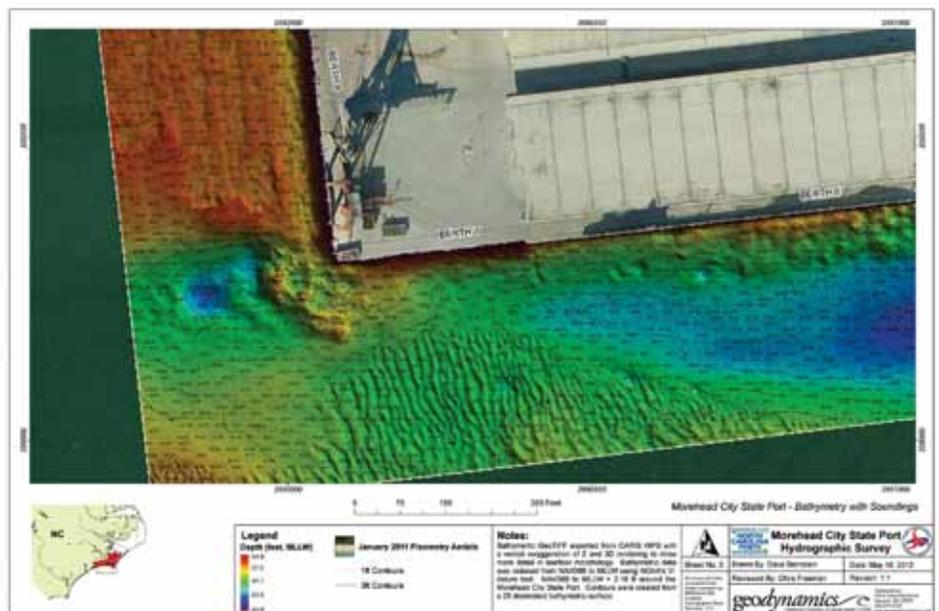
Final data from a high-resolution multibeam sonar survey at the Morehead City Port Terminal. Data were used to assess depths for vessel clearance and to determine rock placement for scour abatement around the berths by Weeks Marine.
