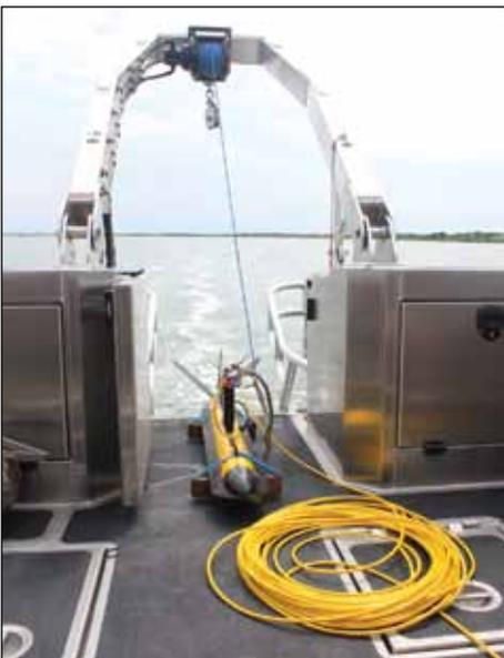
The sidescan being readied for deployment from A-frame.
